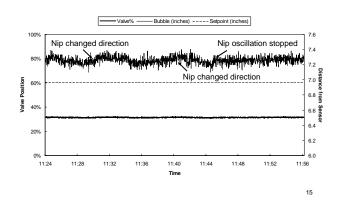
Even slight misalignments in the collapsing frame will move the bubble away from the centerline, resulting in layflat width variation. An easy way to detect this problem is to stop the oscillation and observe what happens to the edges as the roll builds up.
