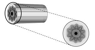
Starred or spoked rolls are a common Transverse Direction wrinkle pattern. It can be caused by baggy film as well as poor winding control.
