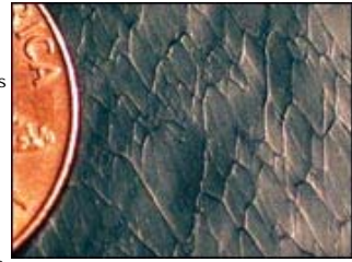
Product samples with problems related to a failure, like this HDPE sheet sample with melt fracture, should be collected and labeled along with material samples from bins and hoppers.
