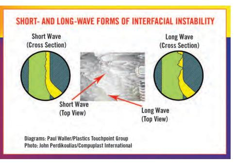
are transmitted through the melt as it exits the die, much as earthquake tremors (also caused by a slip/stick release of pressure in the earth's crust) ripple out from an epicenter.
