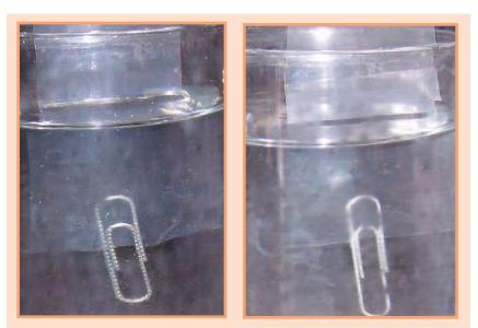
To tell if haze is caused by melt fracture or interfacial instability, immerse a film sample in water and weigh it down with a paper clip. Melt fracture, on the surface, disappears in water; interfacial instability, which is inside the film, doesn't, so the paper clip appears blurry.
