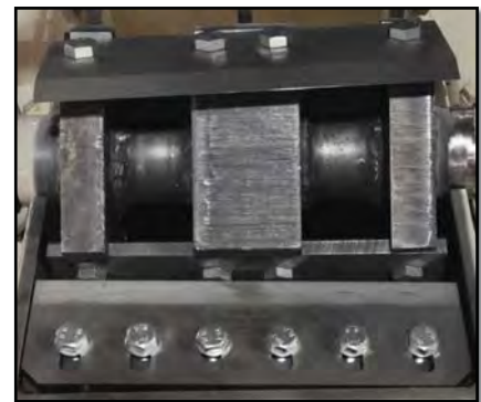
Cutting Chamber Interior
