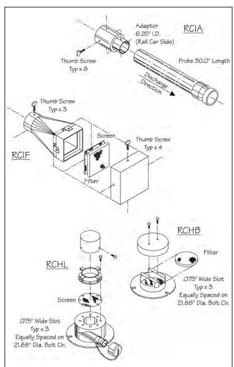
Rail Car Hardware from Process Control Corporation: part of a complete pneumatic conveying system.
