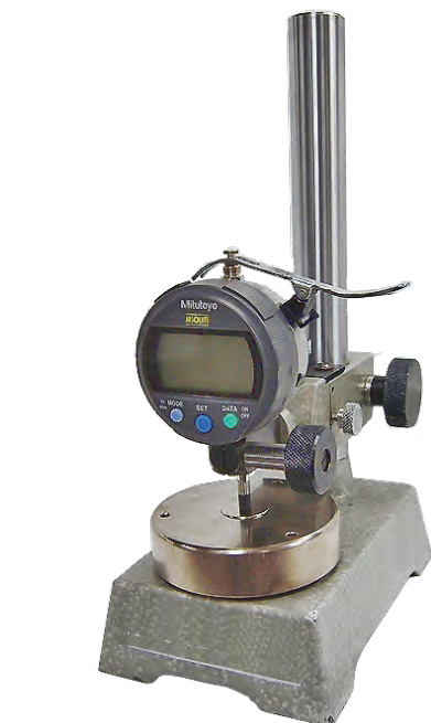
Model 543-392 Battery Powered Digital Indicator. Shown with 7002-10 Dial Gauge Stand upgraded with Parallelism Adjustable Anvil option. Indicator equipped with lift lever and Digimatic™ Serial Output.
