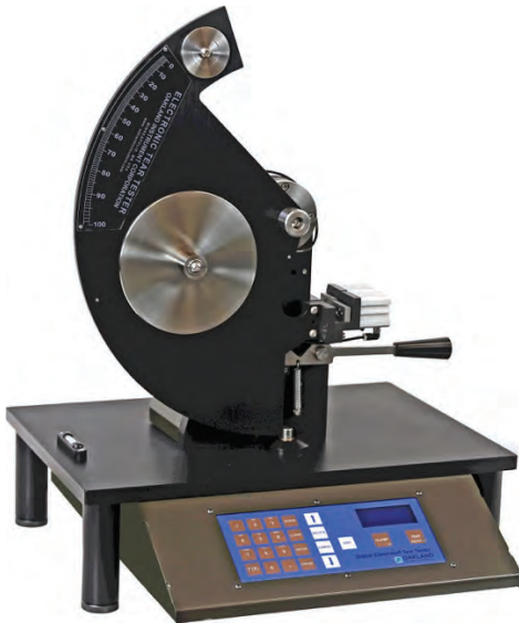
The Model DE-1600-CS Digital Elmendorf Tear Tester with solid Pendulum and 1600 gram Add-Weight for a 1600 gram (15600 mN) Tear measurement capacity. Includes Pneumatic Sample Clamps and Integral Sample Cutting Knife
