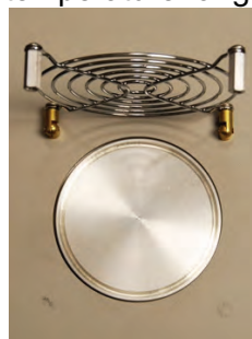
Top-loading Hot Plate with protective flip-up heat shield. Place film sample on top of hot plate for shrinkage testing (Shown at left). Easy to read backlit measurement grid for measuring shrinkage of samples after removing from hot plate (Shown above).
