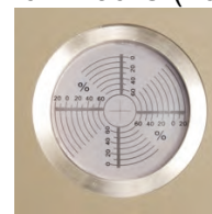
Top-loading Hot Plate with protective flip-up heat shield. Place film sample on top of hot plate for shrinkage testing (Shown at left). Easy to read backlit measurement grid for measuring shrinkage of samples after removing from hot plate (Shown above).
