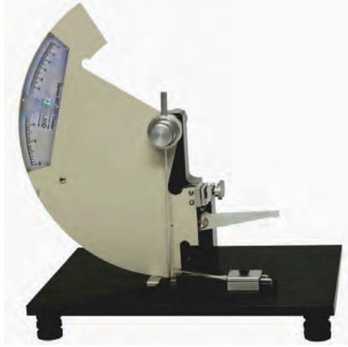
The Model ME-800 Elmendorf Tear Tester with Manual Sample Clamps and Integral Sample Cutting Knife Mechanism
