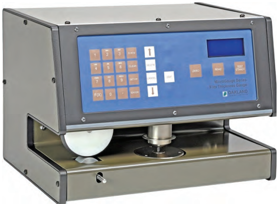
Model MX-1225 Digital MicroGauge Thickness Tester with Isolated C-Frame feature. Gauge equipped with RS-232 Serial Output.
